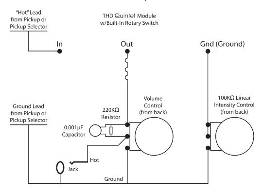
**Typical installation using intensity control**
